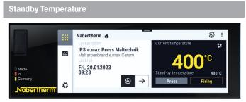
Depending on the furnace model, the standby temperature can be selected for the firing or pressing process and also adjusted individually.
