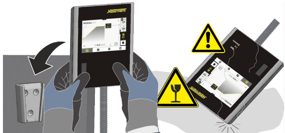
Fig. 33: Place the controller in the holder on the furnace (similar to the picture)
