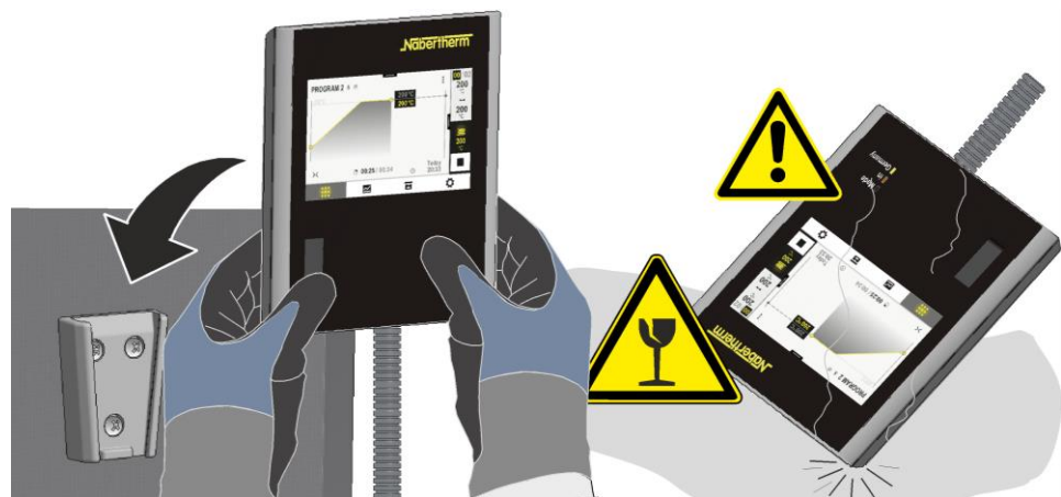
Fig. 21: Place the controller in the holder on the furnace (similar to the picture)
